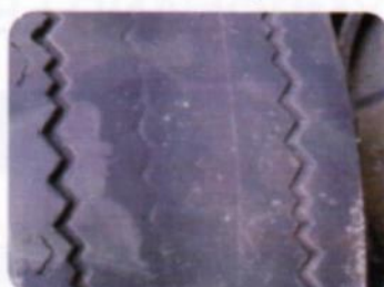
Tread Wear Under high Pressure
