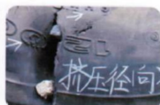
Foreign Material Between Side Wall
