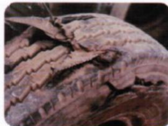
Tyre Crown Impact Blast
