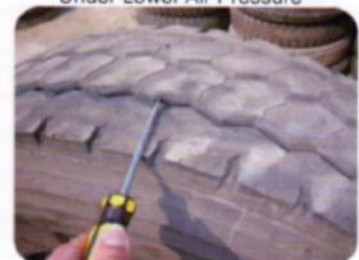
Tyre Crown Abrasion Under Lower Air Pressure
