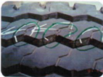
Tyre Crown Pattern Breaking Injury
